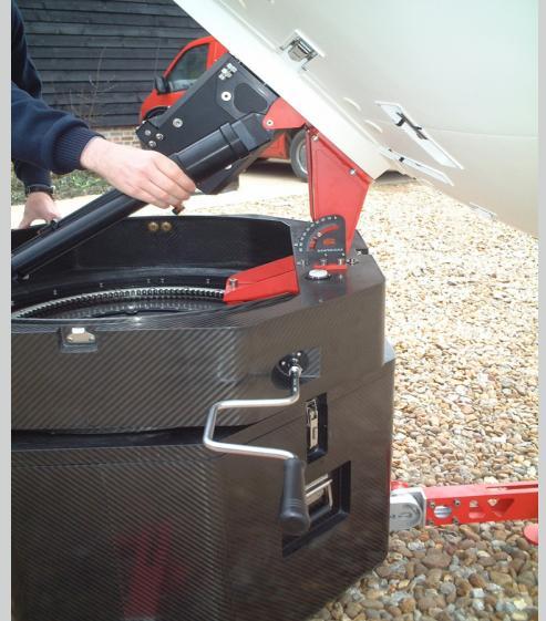
For transportation the FA-180 packs into its own mount which splits into two conveniently sized flight cases for transportation. There are no other cases required.
