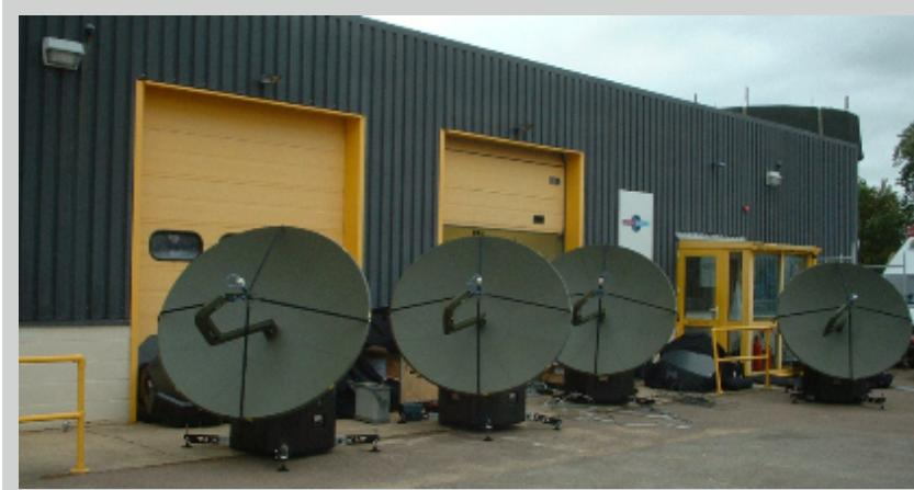
The FA-180 is intended primarily for Satellite News Gathering in C, Ku or K-band, but is equally well suited to any other application requiring a compact rugged antenna which is rapidly deployable with no tools. It includes a multi segmented carbon fibre honeycomb reflector, ensuring light weight and maximum strength with no deformation, even after being reassembled hundreds of times.
