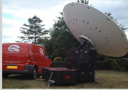
The FA-370 is a compact ultra high gain antenna which can be easily deployed by one person with no tools in less than 30 minutes.
