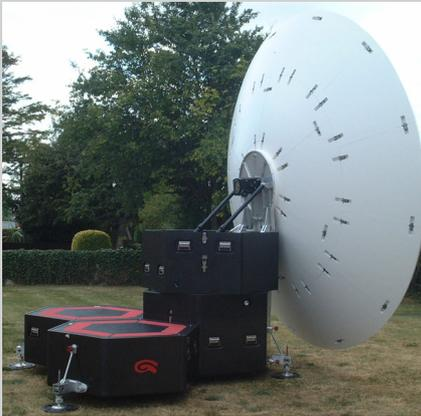
The axially symmetric prime focus feed system was chosen because of its overall compact dimensions and commonality of spare parts. A spares holding of only two petals is all that's required to repair a reflector in case of damage. Compliance with all satellite authority specifications is guaranteed, including side lobe performance better than 29-25 logθ.
